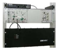
channels in the frequency band 138 - 174 MHz. Daniels MT-4E radios systems support clear or secure (encrypted) P25 and analog voice radio communications. (Secure mode operation is optional.)
